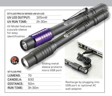
You won't want to be without this sleek, compact penlight that recharges at any USB port or with optional AC wall adaptor. Consistent light output throughout battery life. IPX4 water-resistant. 1 meter impact-resistance tested. Removable pocket clip. UV LED model provides ultraviolet light for detection of fraudulent documents, forensic investigations, or detecting engine or HVAC leaks.
