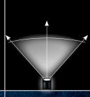
OUTPUT: 120 lumens INTENSITY: 900 candela **BEAM DISTANCE:** 60 meters RUN TIME: 3 hours 30 min **SIZE:**  $1.75'' \times 2.70'' \times 2.40''$  (4.45 × 6.85 × 6.09 cm) **WEIGHT:** 5.5 oz (156 g) **COLOR:** Yellow
