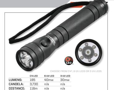
Three lighting modes let you choose exactly the brightness, distance and run time you need. Provides an even beam, along with a piercing hotspot for distance. Unbreakable lens. IPX4-rated for water-resistance. O-ring sealed. 1 meter impactresistance tested.
