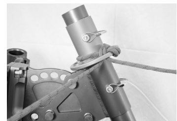
Fig 21 Lash ring on tripod
