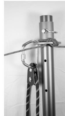
Fig 23 Lash Ring atop of gin pole as main attachment
